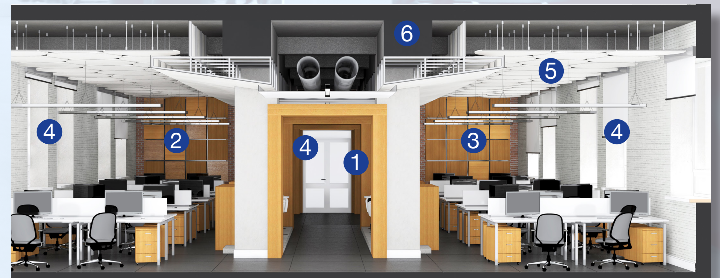
Energy harvesting wireless sensors can monitor building conditions and invoke intelligent control strategies to optimize the use of HVAC and lighting systems in a building.
